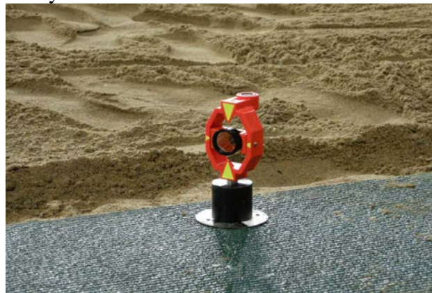
Fig. 4. EDM measurements of markers.
